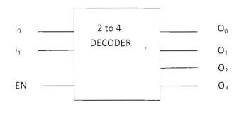
3) (10 points) Implement a 2 to 4 decoder using AND gates and inverters, (you may use 3 input AND Gates). You must show a truth table, boolen equations for each of the four outputs, and then the implementation of the 2 to 4 decoder.
