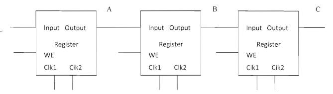
Assume the following signals are applied to the registers above. Draw the signal at point A (output of the first register), point B (output of the second register) and point C (output of the third register). Assume all stored signals are UNKNOWNS at start.
