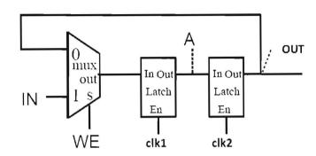
Assume the following signals are applied to the register above. Draw the signal at point A (output of the first latch), the signal at point OUT (output of second latch). Assume A and OUT start at unknown values which are shown below as both a high and a low at the same time with cross hatches drawn between the two values.
