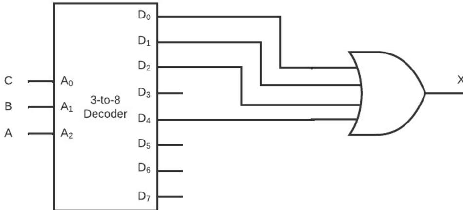
PART B (10 points) How many transistors would you need to implement the circuit above? Assume that the decoder is implemented using canonical sum-of-products equations (no minimization), complemented inputs are provided inside the decoder, and logic gates have no limit on the number of gate inputs.
