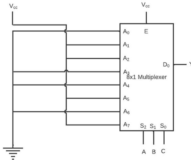
PART D (10 points) How many transistors would you need to implement the circuit above? Assume that the multiplexer is implemented using pass gates and complemented inputs are provided.
