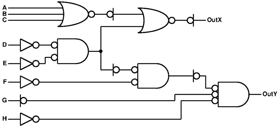
Part A (10 points) Write the output expression for the gate design shown above. Also determine the number of switches used in its implementation.
