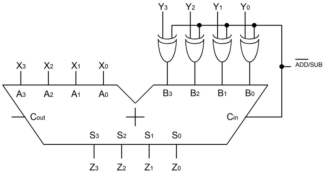
Part C (6 points) Write two Boolean expressions indicating signed two's complement addition and subtraction overflow using inputs  $X_3, Y_3, Z_3$ . These SOP expressions should be true when overflow occurs.
