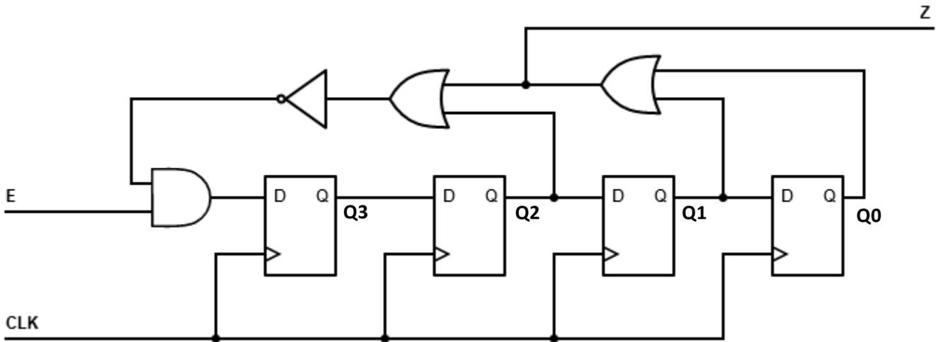
4a) Complete the blank entries in the following transition table based on the state machine above. The state “names” are the same as the state encodings  $Q_3$ - $Q_0$ .
