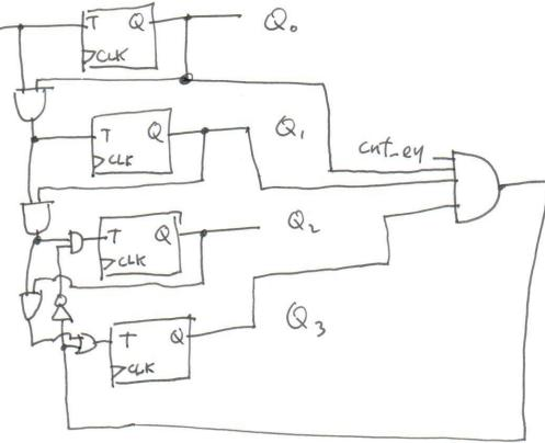
All clk inputs connected to CLK signal.
