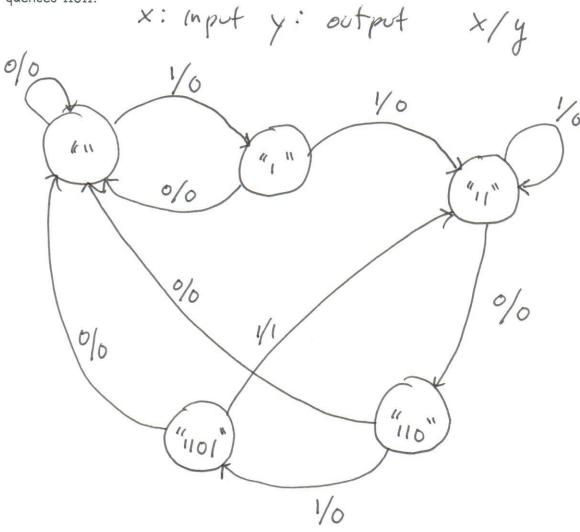
d) (15) Given the following symbolic state state table with input X and output Y, produce a state transition table and find minimized next state and output equations for  $Q_1^+$  and Y only. Use the state assignment where the binary representation ( $Q_2Q_1Q_0$ ) of state variables for state Si = i. You do NOT need to draw a schematic.
