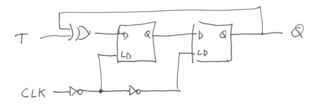
(b) (15) For the given circuit (D Latch and negative edge triggered 7-FF), complete the timing diagram. Note that U and V are initially 0.
