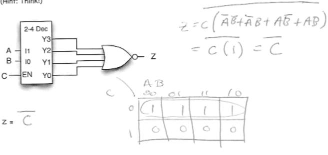
b) (10) Design a 2-4 decoder with enable using 1-2 decoders (as many as you need), and a minimum number of additional gates if necessary. Use the decoder symbol as given, and duplicate as many times as needed. All signals (inputs I<sub>1:0</sub>, EN, and outputs Y<sub>3:0</sub>) must be labeled correctly.
