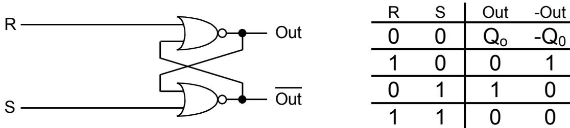
Part B (7 points) Expand the RS latch to a transparent latch and complete the truth table. Use only basic gates (AND, OR, NAND, NOR, and NOT). Label the inputs and output. Also complete the behavior table.
