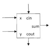
b) (10 Points) Using four of the full adder blocks shown above to the right, show how four of them would be used to implement a four bit adder that would be able to add/subtract two four bit numbers. Your inputs are X3, X2, X1, X0, Y3, Y2, Y1, Y0, add/sub, S3, S2, S1, S0. You may use any additional logic gate types you want. Draw your hardware diagram below:
