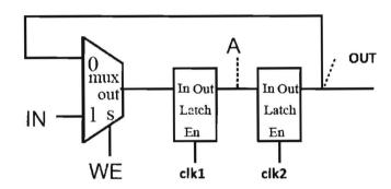
Assume the following signals are applied to the register above. Draw the signal at point A (output of the first latch), the signal at point OUT (output of second latch). Assume A and OUT start at logic unknown values.
