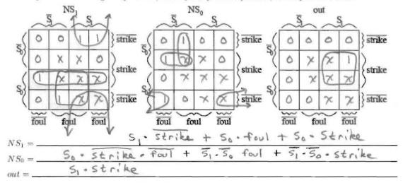
Part C Implement this state machine using your expression from part B, plus two register cells. Use an icon for a one bit register cell. You do not have to show the implementation of a register here. Your logic should be simplified.
