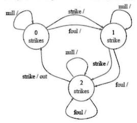
Part A Using the state diagram above, complete the state table for this diagram. The inputs are strike, foul, and state bits  $S_1$  and  $S_0$ . The outputs are next state bits  $NS_1$  and  $NS_0$ , and out.
