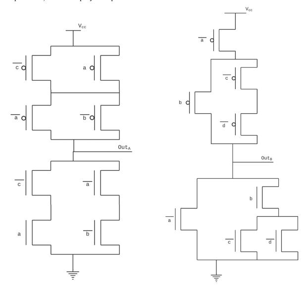
$$Out_A = \underline{\phantom{a}}(c + \overline{a}) \cdot (a + b)\underline{\phantom{a}}$$
