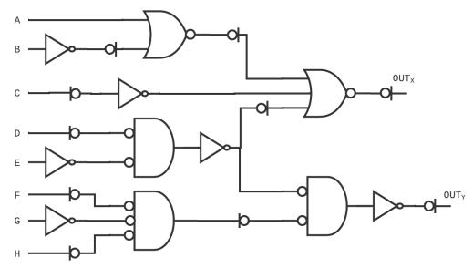
Part A (10 points) Write the output expression for the gate design shown above. Also determine the number of transistors used in its implementation.
